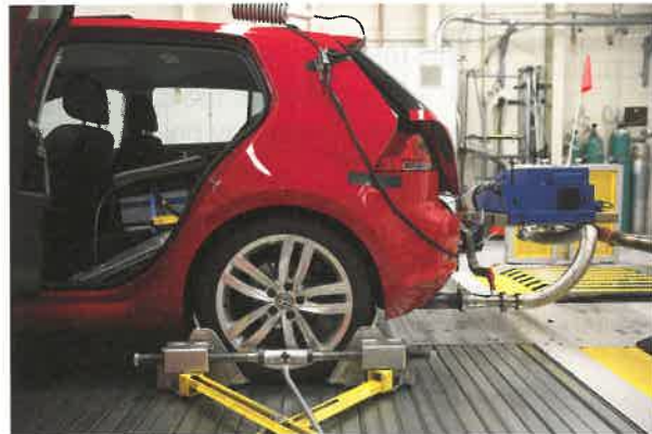
▲ A VW vehicle being tested for emissions
